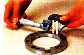
Measuring distance between holes
