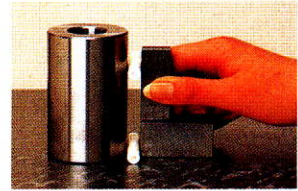
Checking right angle
